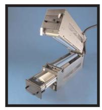
advanced 4 and 6-roll assemblies allow the top-half of the cleaner to open and the tape-rolls to slide out on drawers. This greatly facilitates tape maintenance and web threading. The HexClam is available to 24" and the QuadClam for 30" to 60" widths. Both are constructed of stainless steel and aluminum for strength and are equipped with a static neutralizing bar and pneumatic cylinder to separate tape rolls from CCRs.
