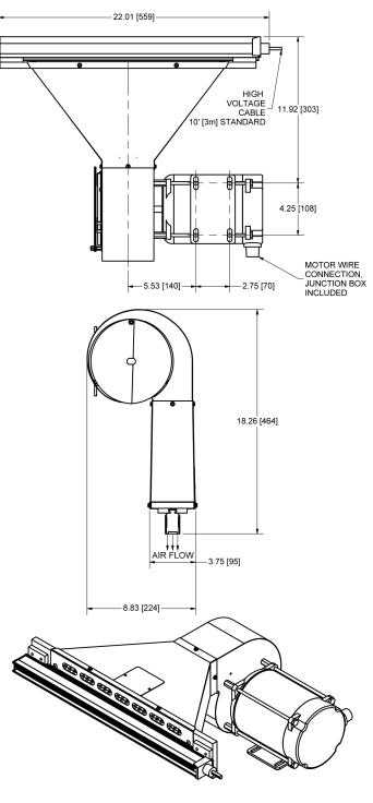
The IQ Power Fantom HL Blower should not be mounted with the motor shaft vertically upward.
