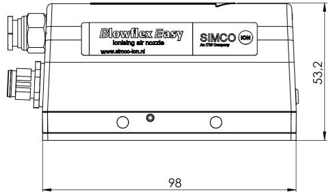
Simco offers Blowflex Easy devices with nozzles for a wide range of applications. If there is no suitable device, you can assemble your own combination of Blowflex Easy Basic and a suitable nozzle. The Blowflex Easy Basic has a 1/4" BSPP air outlet.
